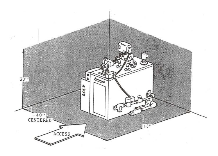
Select a location for mounting the Steam Generator that is accesible for the installation and service. The above service area indicates the minimum space required for convienient access.
