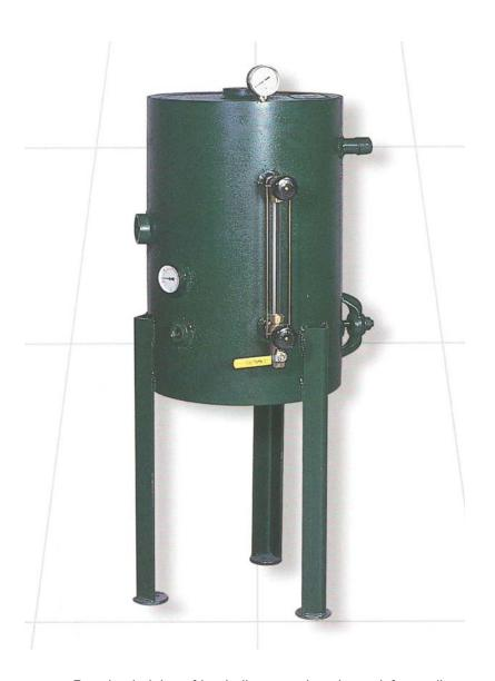
Permits draining of hot boiler water into the tank for cooling before it is dumped into drainage system. Allows HC blowdown system to comply with codes that prohibit the discharge of water exceeding 140°F.
